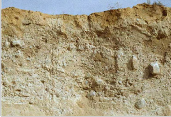
Figure 3.13: Glacial till. Note the mixture of grain sizes from large rocks to fine sands, silts, and clays that indicate no reworking by water. (from http://nesoil.com/images/tillcut.htm , 2010).
